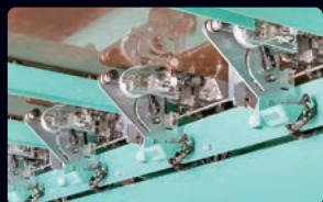
Smart Bobbin Changer It takes the SBC only 6 seconds to replace the bobbins for all heads. Raising production efficiency to a great extent!!
