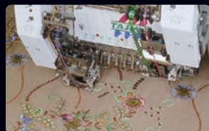
Sequin Device III [Twin Type] <PAT> A device for embroidering 2 different sequins by freely switching them at high revolving speed
