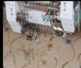
Sequin Device III [Twin Type] <PAT> Embroidering 2 different sequins by freely switching them at high speed
