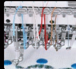
Multi cording Device Embroidering 6 various types/colors of cords
